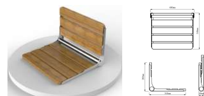
Product: Showering Seat Item No.: CF-007 Materials: SU304 Stainless Steel+ Red Oak+POM Weight/pc: 3.9kg Dimension of Product: 40*340*268 (unfolded) 40*84*340 (closed)mm
