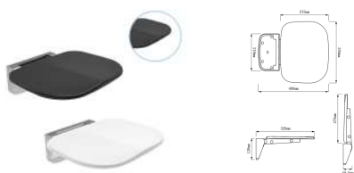
Product: Showering Seat Item No.: CF-006-1 (white) CF-006-2 (black) Materials: FU Urea Formaldehyde+ Nylon+Silica Gel Weight/pc: 2.5kg Dimension of Product: 350*40*15 (unfolded) 350*50*392 (closed)mm
